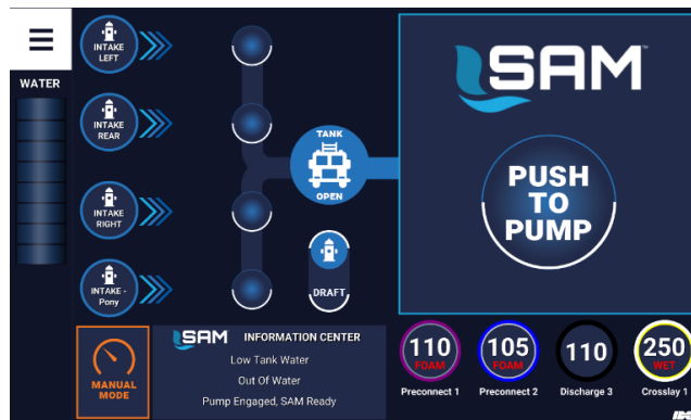
Figure 14. Activating A CAFS FOAM ONLY Quickset
