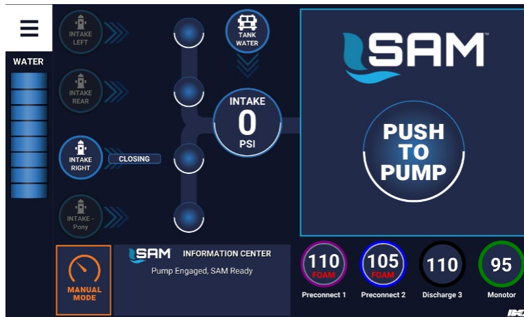
Figure 2. Activating A Foam Quickset
