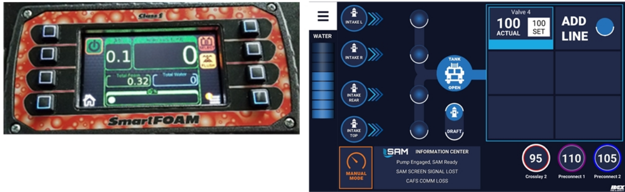
Figure 3. SmartFOAM With SAM Quickset Activated
