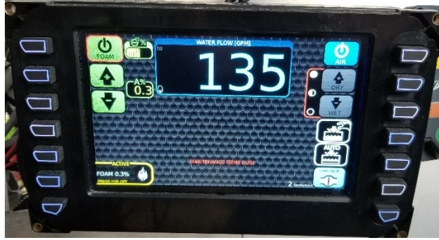
Figure 20. SmartCAFS Display With SAM FOAM ONLY Bubble Activated
