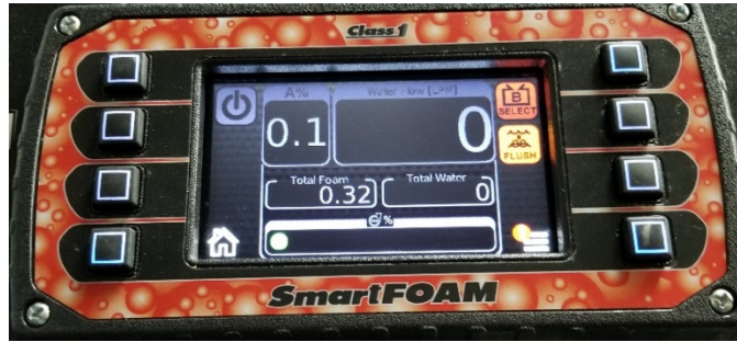
Figure 8. SmartFOAM Display With No FOAM Discharges Active
