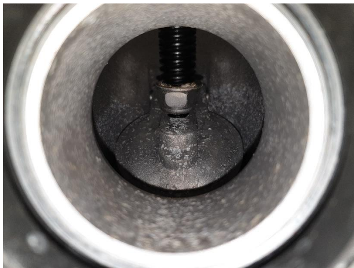
Screw down valve, view through the connector showing the spindle with the Nyloc nut and washer fitted to the end of the spindle.
