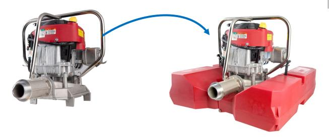
**7.3** Secure the engine to the float by pulling the flexible straps and hooking into the keeper on the frame. There are two flexible straps, one on either side of the frame.
