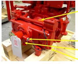
Bearing housing oil level dipstick and filling aperture.
